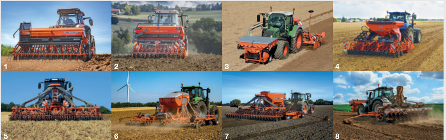
1. Mounted mechanical - 2. Integrated mechanical - 3. With front hopper - 4. Integrated pneumatic - 5. Trailed pneumatic - 6. Mounted for min-till seeding - 7. Trailed for min-till seeding - 8. Precision seed drills
